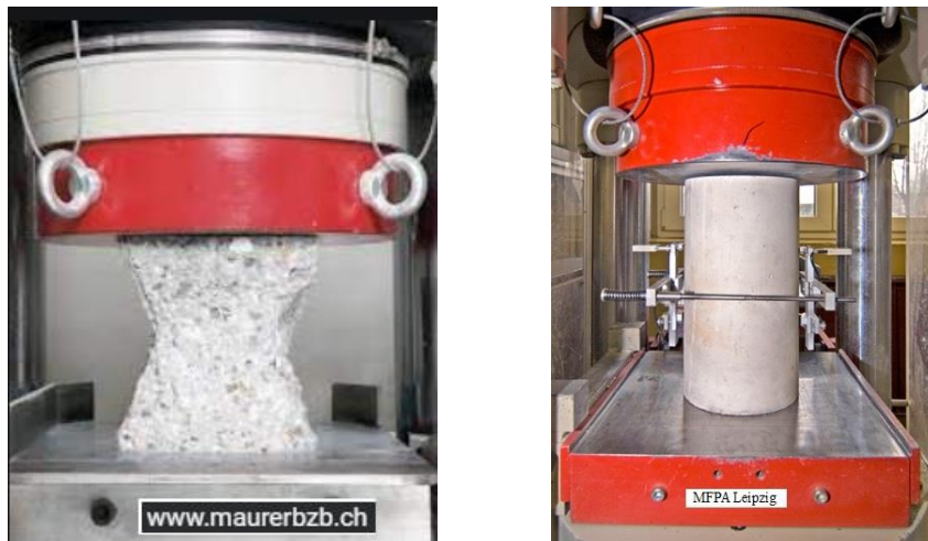
Fig.5-2: Test rig and test specimens of concrete
