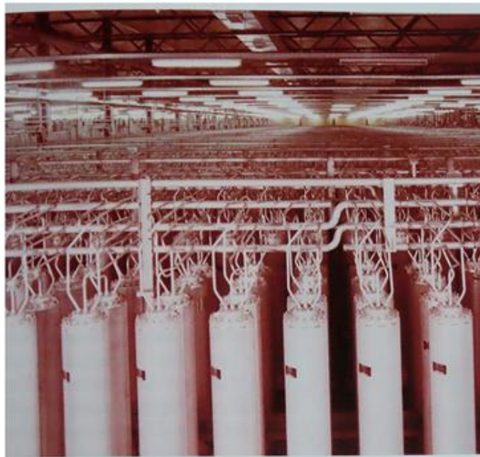
Uranium enrichment in Gas-Ultra-Centrifuges (metal, CFRP). Separation of U 235 from U 238
