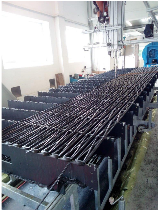
Fig.4-5: CFRP truss work production using a special strand placement (winding) technique and the fabricated bridge [BaltiCo GmbH, July 2020]. Thanks Dirk 25 m bicycle and pedestrian bridge made of CFRP in Sassnitz was installed, which was easier than usual due to the weight of just 1.4 tons of a single segment and took place within a single day. BaliCo Portfolio: Lattice masts, functionalized modular cabin plate elements, bridges, girders, lattice masts, telescopic towers, rotor blades.
