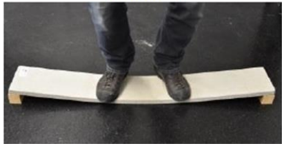
Fig.4-12: Application of pre-tension. The concrete is compression-activated, which massively increases the stiffness of the component, carbon fiber strength can be fully utilized. (center) Stiffness for service loads remains for CPC pre-stressed. (right) Permanent deformation for the slack reinforcement (Stahlarmierung, schlaff) due to the stretched steel reinforcement
