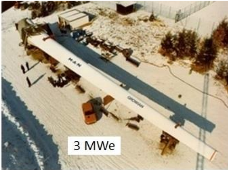
GROWIAN tested at IABG, 1980, GFRP shell
