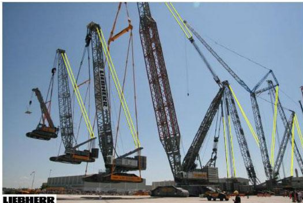
Fig. 4-7: CFRP tension members made of continuous loops for cranes, since 2003 [Liebherr with with the EMPA Spin-Off Company Carbo-Link]
