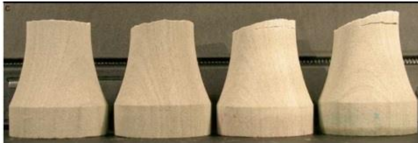
Fig.6.6-2 Sandstone: Fracture pictures of Berea sandstone from [Lan19].
