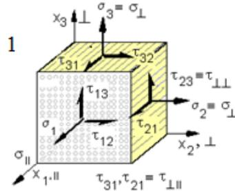
Fig. 3: FMC-based strength failure conditions [Cun12, 13]
