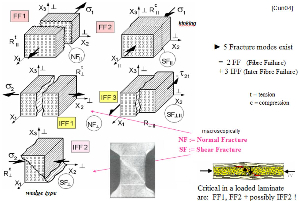
Fig. 2: Fracture failure modes of UD material
