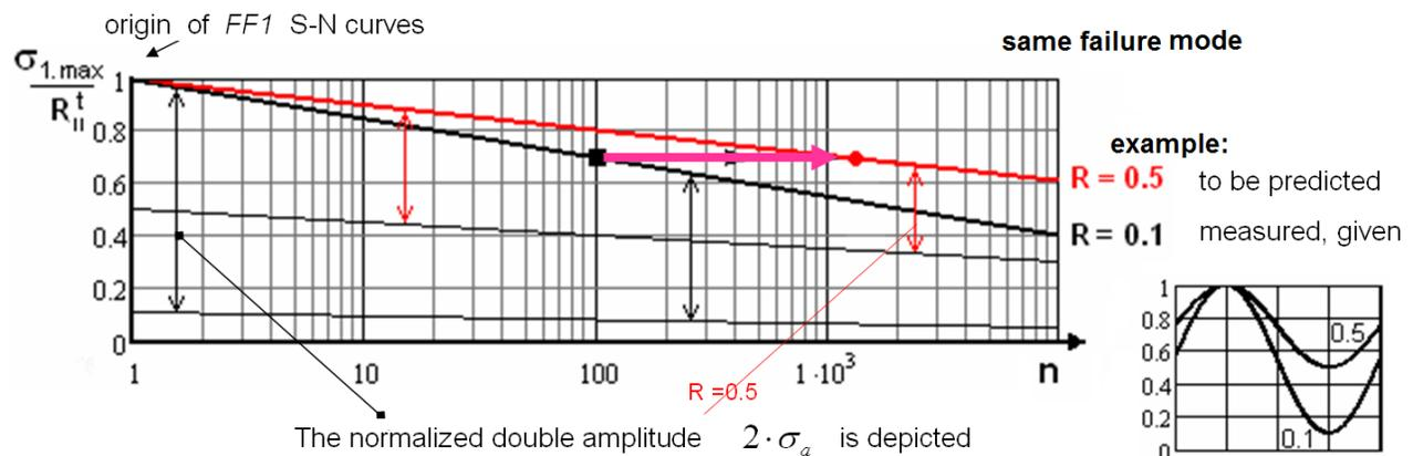
Fig. 7: Schematic S-N curve prediction by using the strain energy equivalence principle
