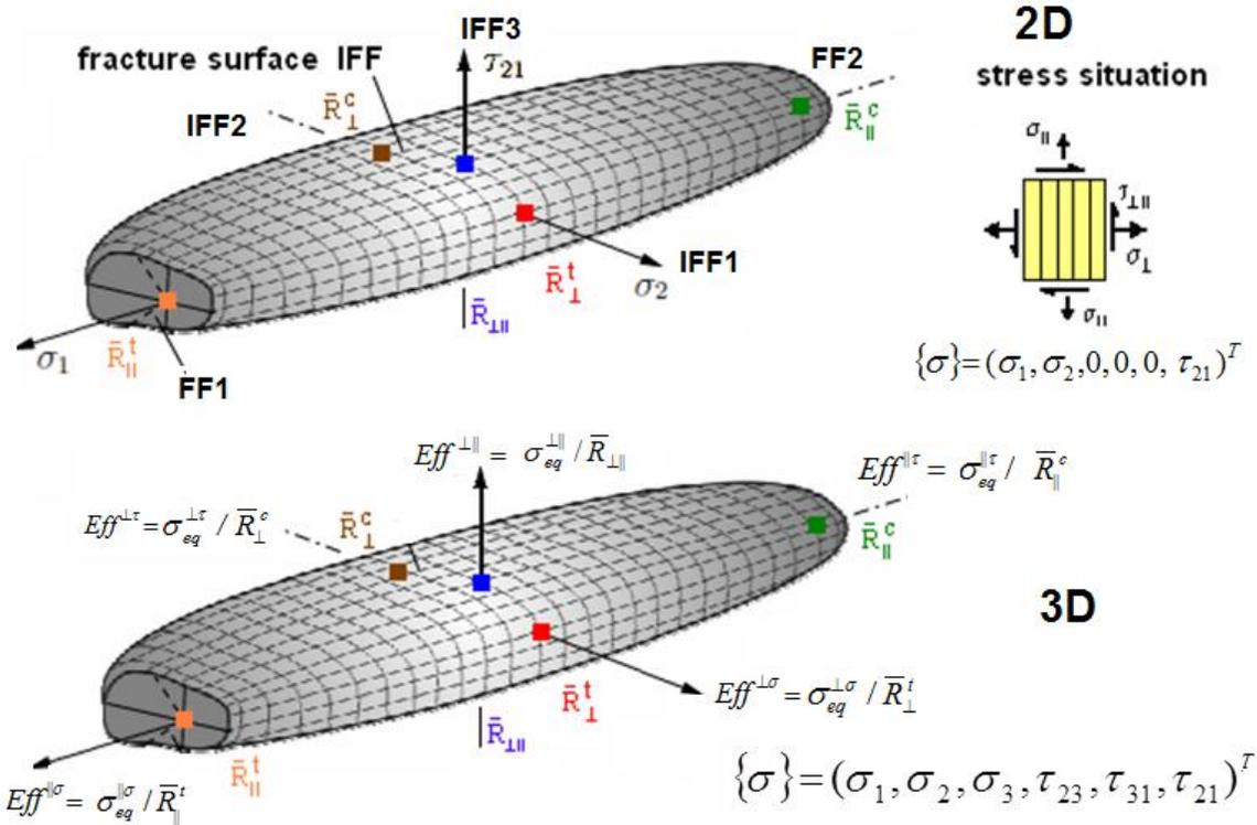
Fig. 4: 2D and 3D failure surface of the FMC-based strength failure conditions
