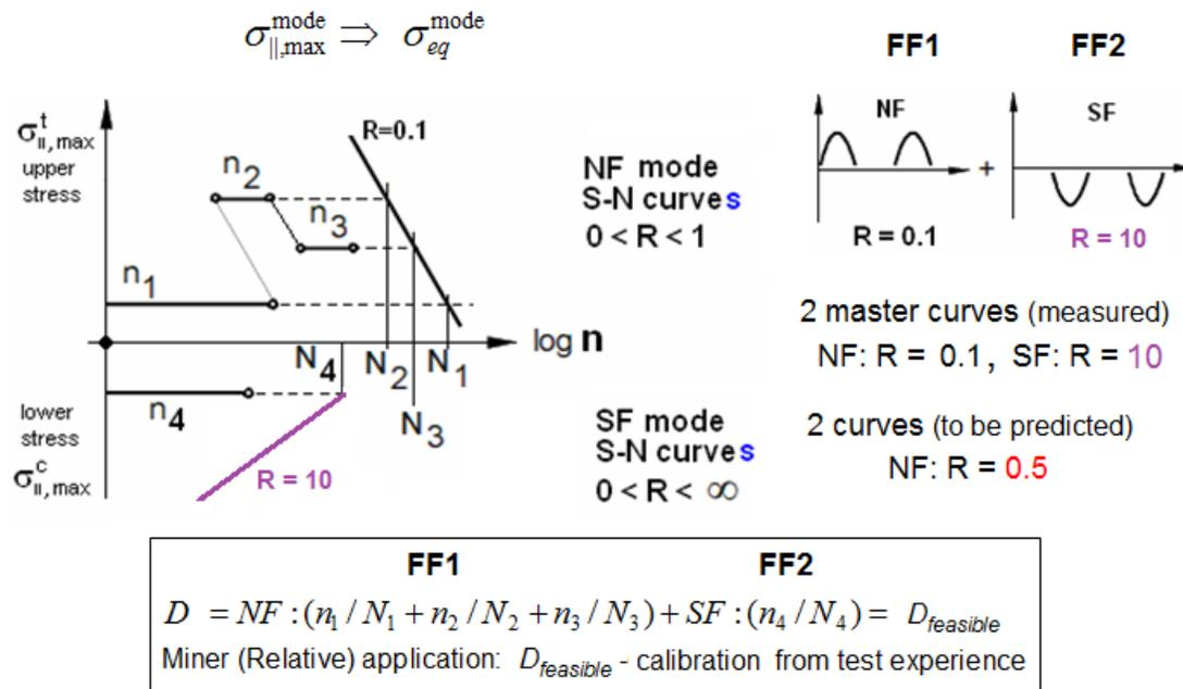
Fig. 9: Schematic application of the method for the two FF modes
