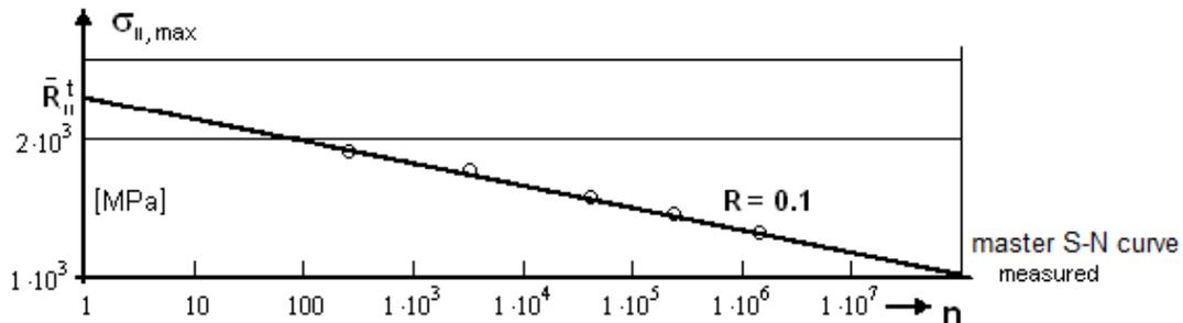
Fig. 6: Modeling of the mode-representative master S-N curve
