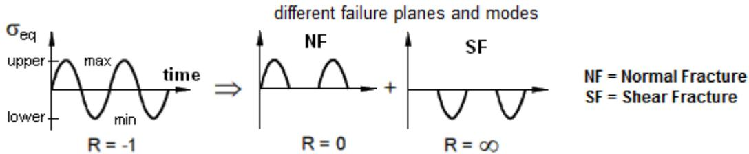
Fig. 5: Novel modeling of loading cycles
