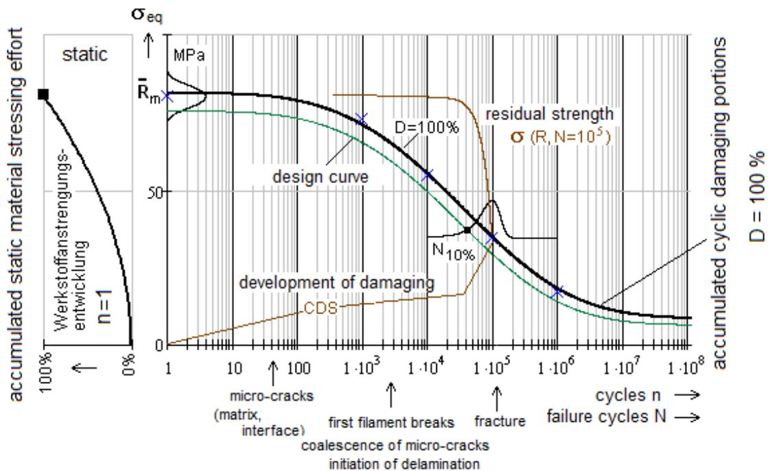
Fig. 1: Notions and development of damaging for a distinct fracture cycle number  $N=10^5$  and stress ratio  $R = \sigma_{\min} / \sigma_{\max}$  of the envisaged fiber failure mode,  $D$  = sum of accumulated damaging portions, CDS= characteristic damaging state; material stressing effort (“Werkstoff-Anstrengung”)
