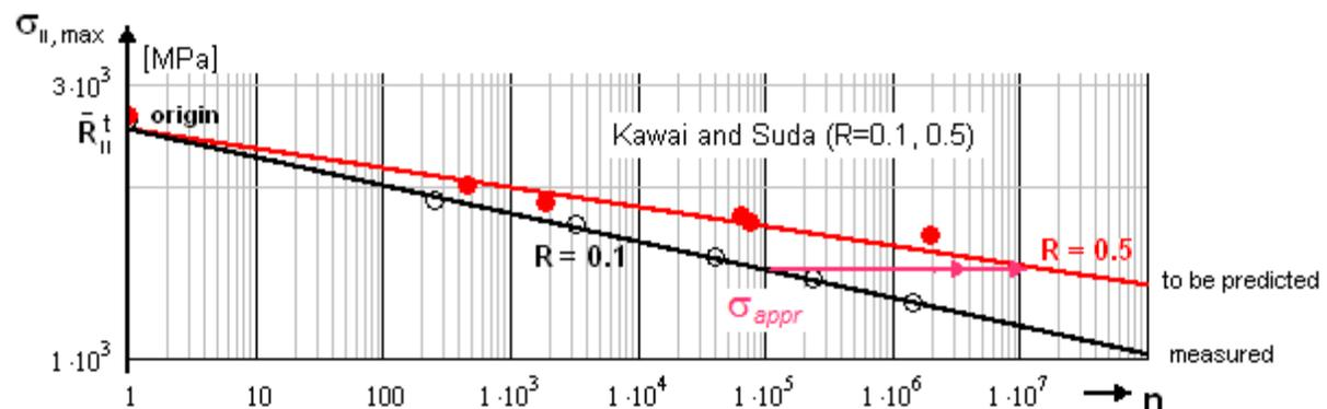
Fig. 8: Prediction of mode S-N curves from a mode-representative master curve
