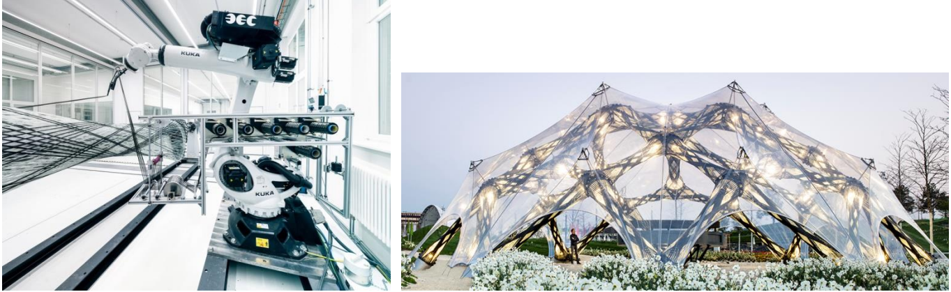
Fig.5: BUGA-Heilbronn. Roving-placing robot machine (left), art-work and load-carrying structure (right) [Knippers, Koslowski ITKE and Menges CD Uni Stuttgart]
