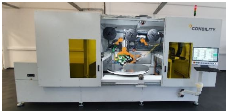
2D Tape Placement Machine with integrated Laser System
