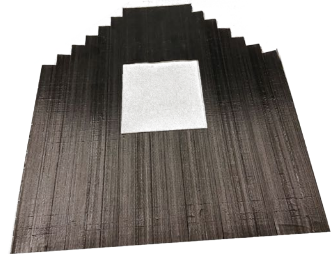
Tailored blanks with / without cut outs
