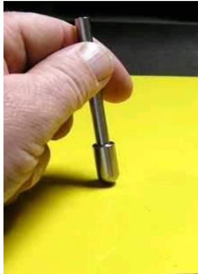
Manual Tap Test Extremely simple NDT instrument pocket size, ultra low cost available everywhere
