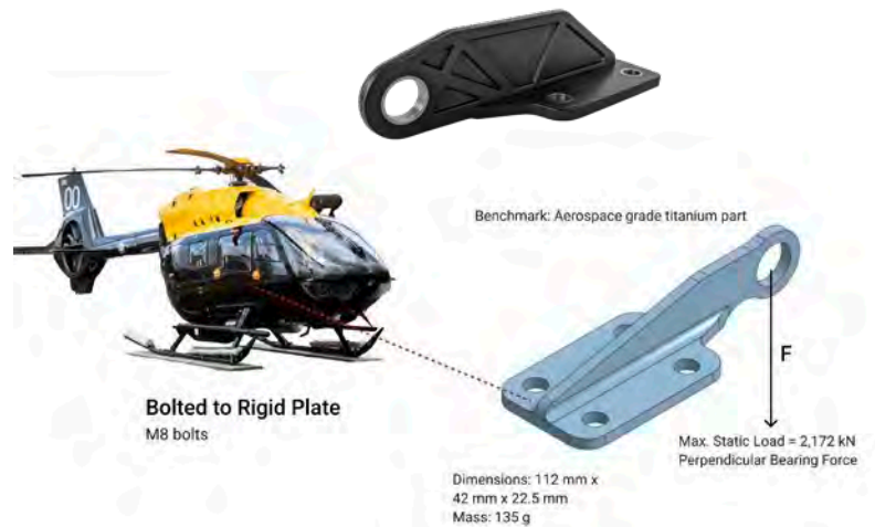
Helicopter hinge in benchmark steel (above) and printed/moulded CFRTP (below)
