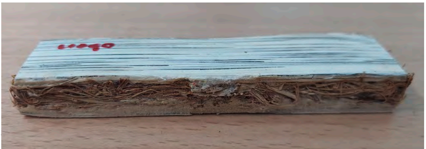
Finished sandwich test specimen
