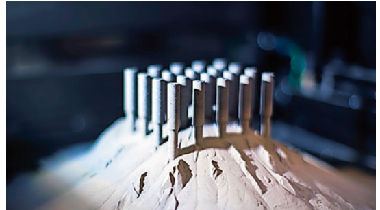
Cylindrical test specimens manufactured with L-PBF near net shape
