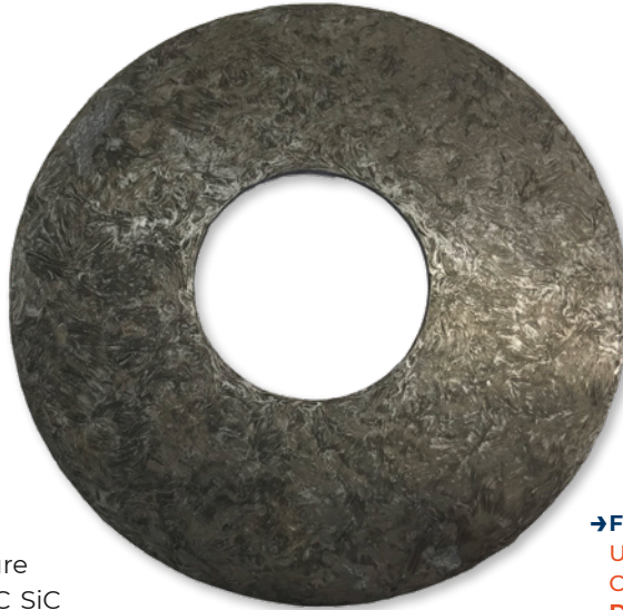
Fig. 2: DC/C-SiC-Demonstrator (Øa = 130 mm Øi = 50 mm in CFRP condition)
