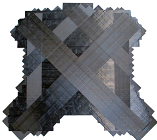
Left: Stack manufactured using a VRA
