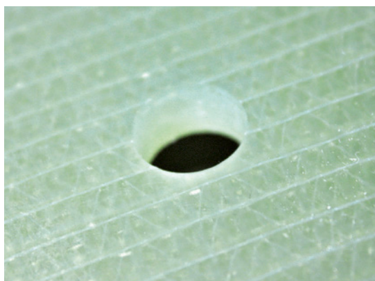
With the HEXA CUT® Eco product line circular milled hole in the reworked glass fiber based automotive leaf spring
