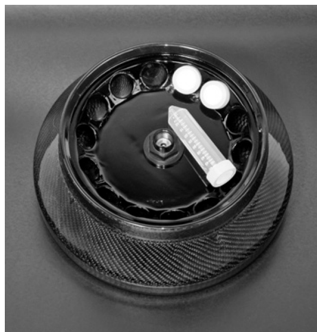
Robot-made laboratory centrifuge made of Gerster Drapfix and spiral mesh
