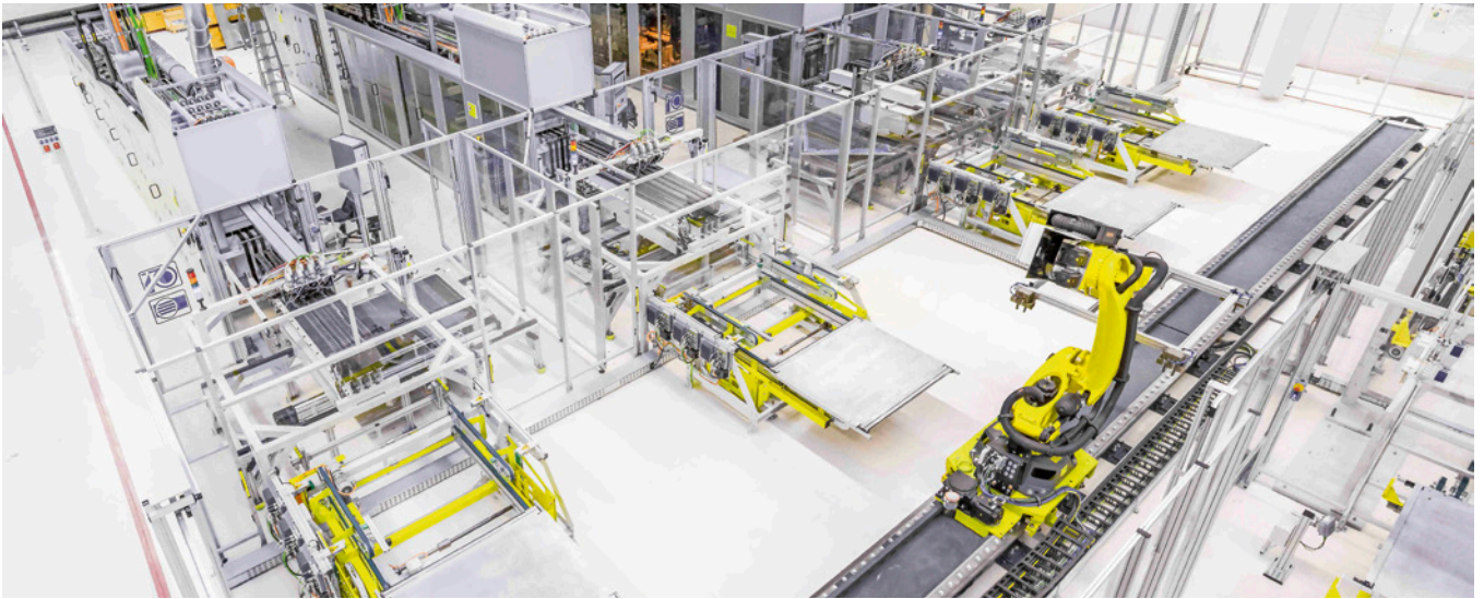
Four VRAs integrated into a fully automated large-scale production line
