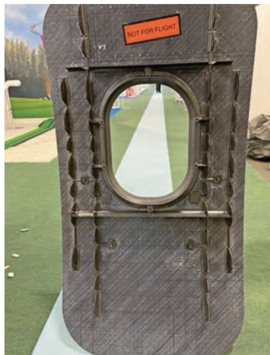
Light for flight: Airbus NMB outer door skin
