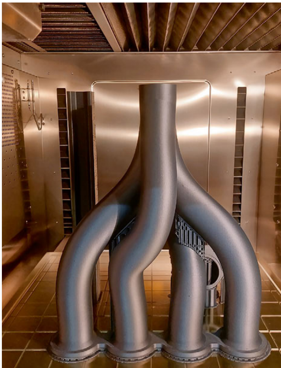
Fig. 1: Industrial Roboze additive manufacturing system for the fabrication of Carbon-PEEK components with complex engineered architectures
