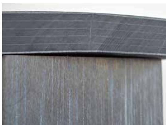
Spar cap section made from pultruded planks (above) and from Magic Flow UD fabric (below)
