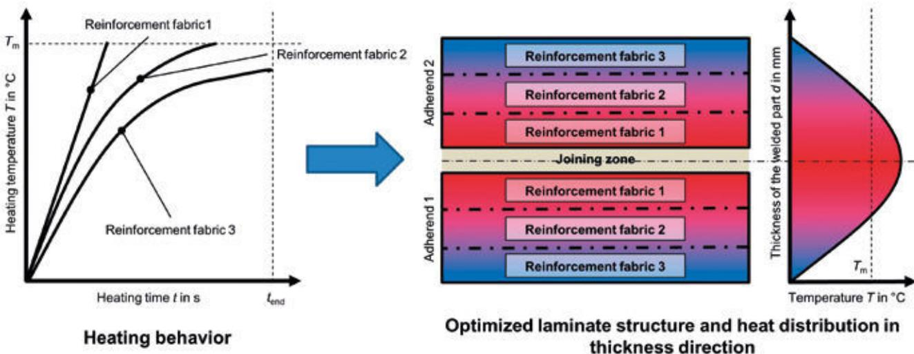
Fig. 1: Optimization of the laminate structure regarding higher welding speeds after heating-up tests of several reinforcement fabrics
