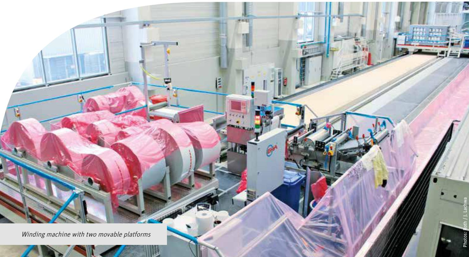
Winding machine with two movable platforms
