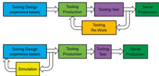
Fig. 1: Tooling design process (top: original approach without simulation; bottom: new approach including MPS)
