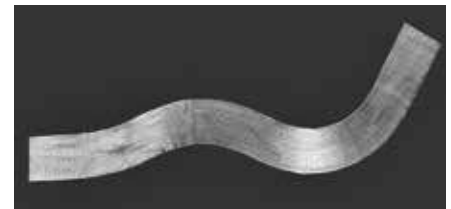
Curvature of the continuous shape ribbon can take any direction, also S-shapes
