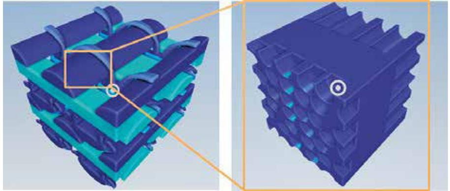
*Fig. 3: Left: Zooming in makes it possible to view the material stress at mesoscopic scale (textile). Right: By zooming in again the material can be viewed at microscopic scale (fibres/matrix) at the same point in the loading process.*
