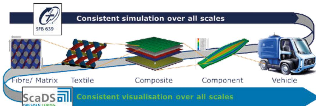
Fig. 1: Multi-scale concept – Simulation and visualisation of material behaviour from individual fibre to overall vehicle.
