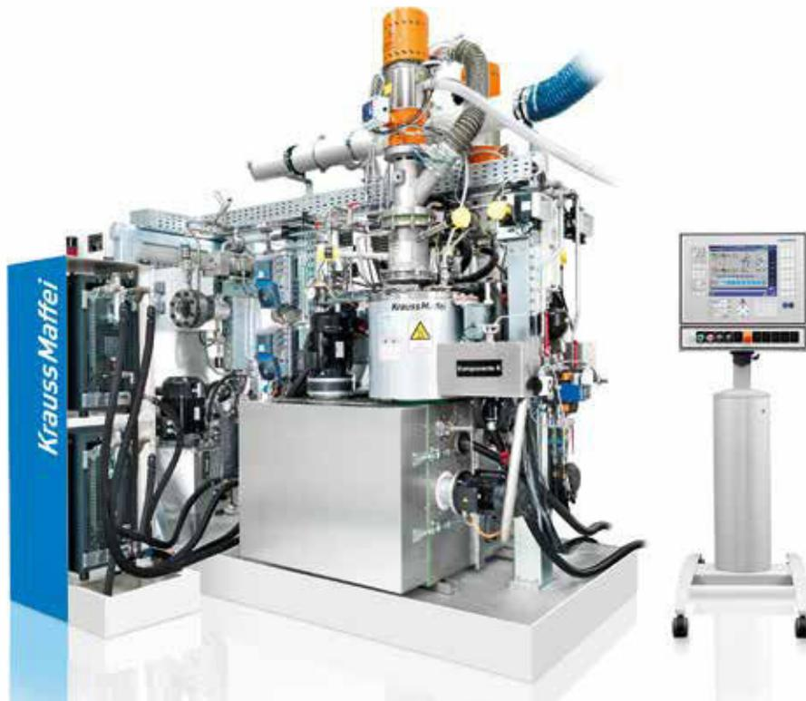
*The new RimStar 8/8 T-RTM metering system enables on-demand melting of the caprolactam components.*
