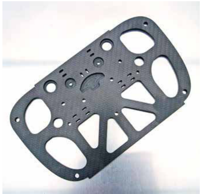
Formula Student Lenkrad in Composite-Bauweise, konstruiert in Solidworks, CNC-Programmerstellung mit HSMWorks Composite "Formula Student" steering wheel designed in Solidworks, CNC programming with HSMWorks
