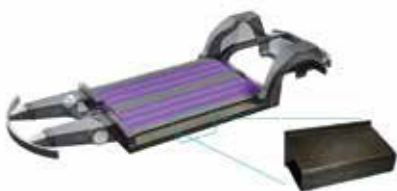
Floor module with hydrogen tanks
