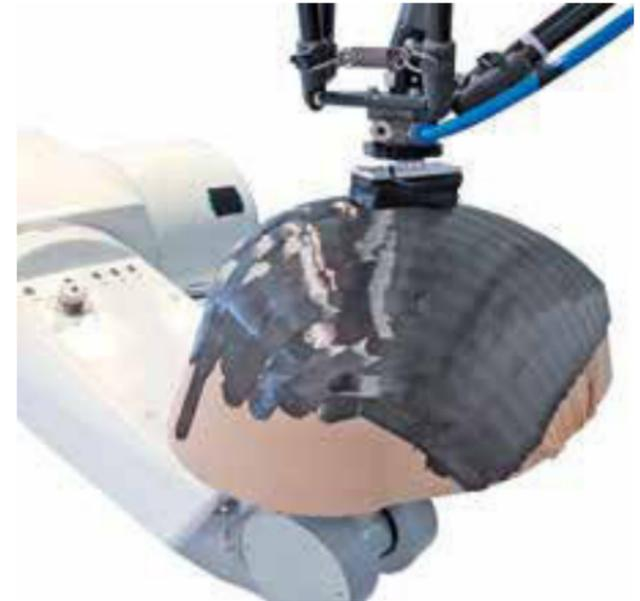
*Additive placement of fiber patches*
