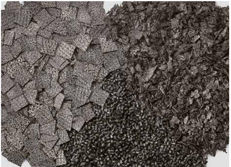
Tenax®-E ThermoPlastic Recycling Solutions (Compound, Chips und Crushed)
