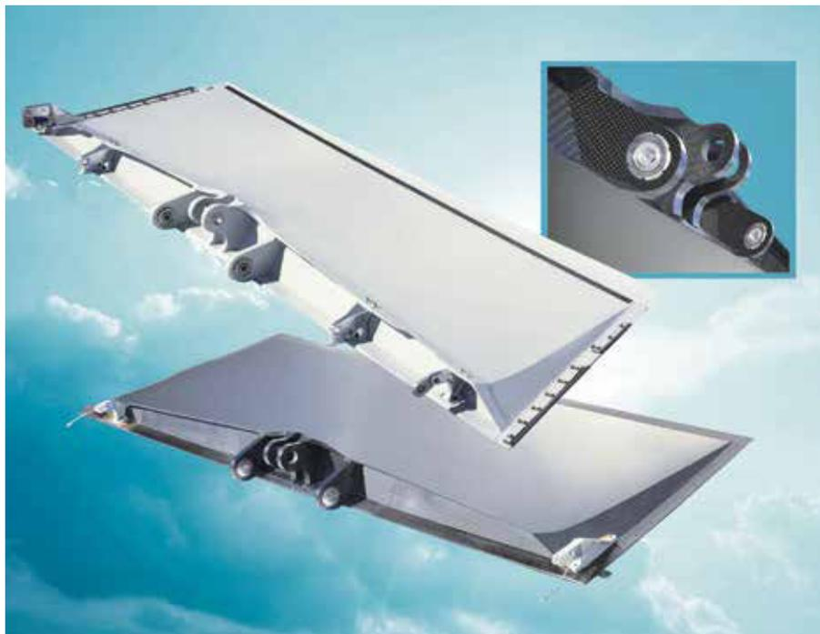
*Center hinge fitting for Airbus A330/340*
