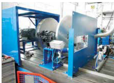
Fig. 1: Self designed dynamometer for high performance friction studies (with a steel fly wheel and a 1 m ø steel brake disc)
