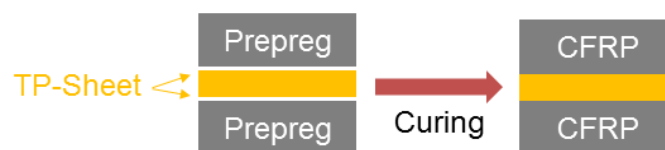
Figure 4. “Perfect” welding process (schematic), TS/TP/TS type joint.
