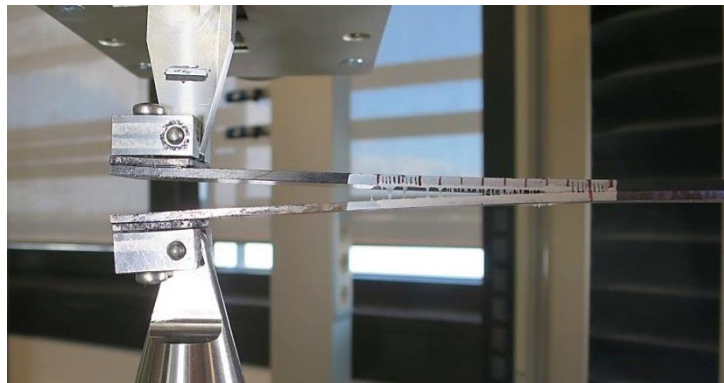
Figure 4. DCB test with specimen out of CFRTP laminate (top) and steel (bottom)
