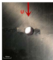
Figure 9. The macro contour of FHC structure with stacking sequence [45/0/-45/90]_{2s} under static compression
