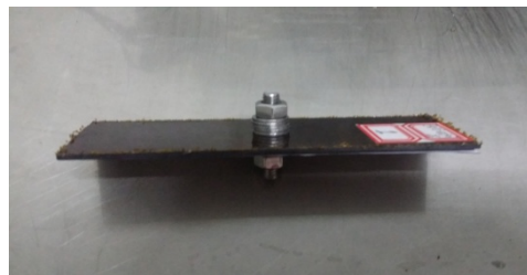
Figure 2. The filled-hole structure specimen with stacking sequence [45/0/45/90] 2s
