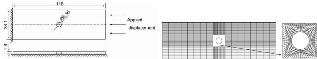
Figure 3. FHC specimen and mesh model with stacking sequence [45/0/-45/90]_{2s}
