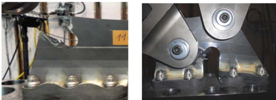
Figure 12. Failure modes: net section (left) and bearing (right). (source SKF Aerospace)
