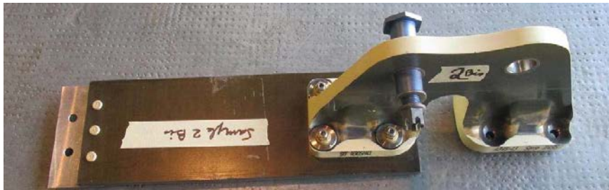
Figure 13. Example of specimen for lightning strike test. (source: Airbus)
