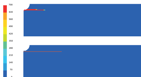
Figure 1. Microcracking computation with mesomodel former (at the top) and new approach (below)
