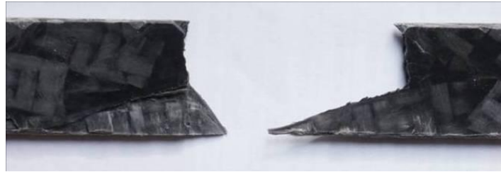
Figure 7. Fracture faces of recycled tensile specimen.
