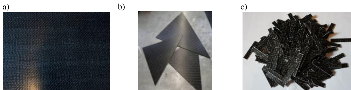
Figure 1. a) Initial pre-consolidated laminate, b) Production scrap, c) aggregates.
