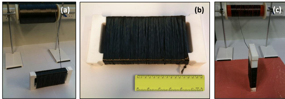
Figure 2. Photographs of (a) as-received fibres winding, (b) as-received fibres wound with scale and (c) bi catalyst precursor deposited carbon fibres.
