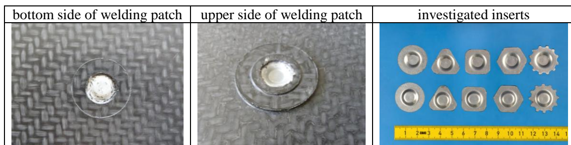
Figure 10. Investigated welding patches and insert geometrics.
