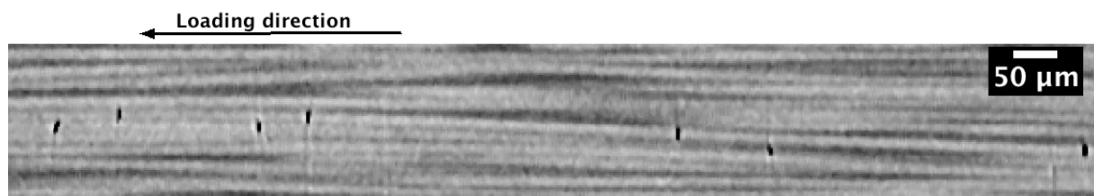
Figure 4. Multiple breaks along the same fibre observed one second before failure.
