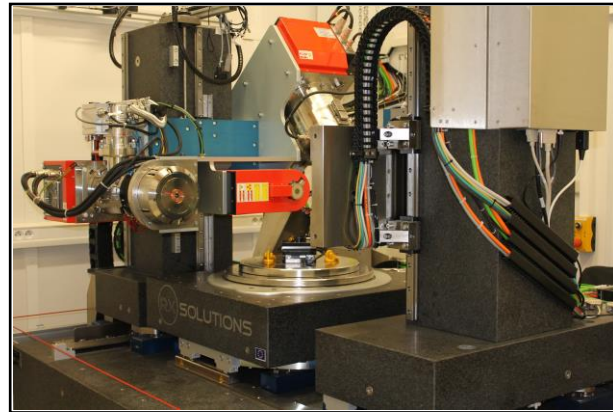
Figure 2. RX Solution® X-Ray micro Computed Tomography facility – available at the Pprime institute
