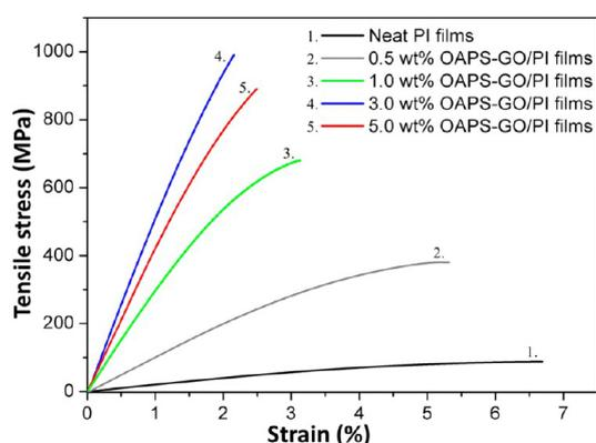
**Figure 1.** Stress–strain curves of neat PI films and OAPS-GO/PI films with various amounts of OAPS-GO.
