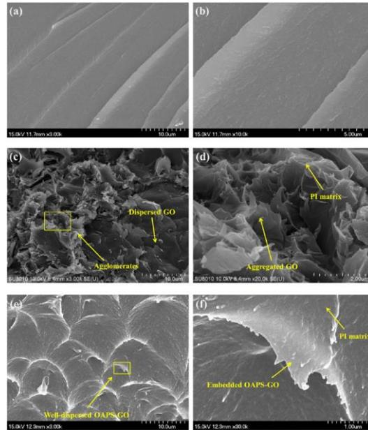
**Figure 2.** SEM images of fractured surface of (a) neat PI ( $\times 3k$ ), (b) neat PI ( $\times 10k$ ), (c) 3.0 wt % GO/PI film ( $\times 3k$ ) and, (d) 3.0 wt % GO/PI film ( $\times 20k$ ), (e) 3.0 wt % OAPS-GO/PI film ( $\times 10k$ ), and, (f) 3.0 wt % OAPS-GO/PI film ( $\times 30k$ ).
