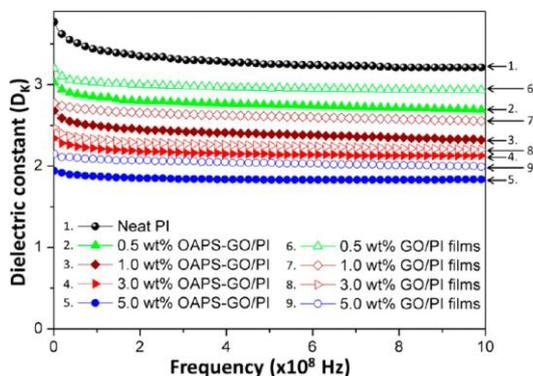
**Figure 3.** Dielectric constant as a function of frequency for neat PI films, OAPS-GO/PI films, and GO/PI films.
