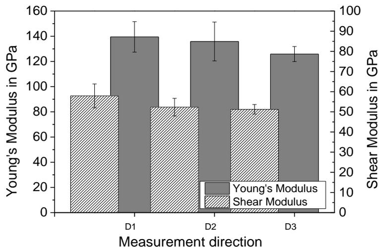
**Figure 3.** Measured Young's Modulus (E) and Shear Modulus (G) (Directions: D1 = direction of infiltration, D2+D3 = perpendicular to infiltration direction)
