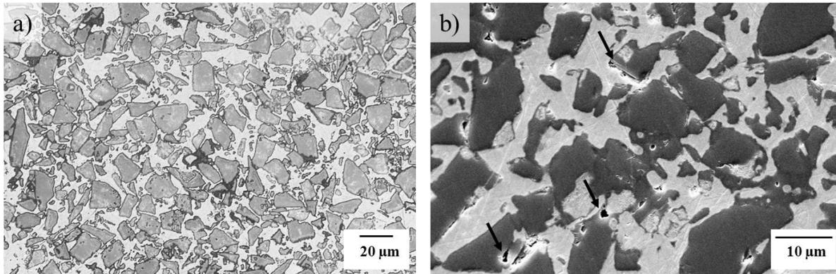
**Figure 2.** Microstructure of the Cu-SiC-Composite (500x) showing a homogenous distribution of the SiC-Phase inside the composite and porosity at the Cu/SiC-Interface (SEM, 5000x)
