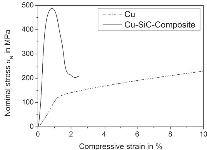
**Figure 4.** Exemplary stress-compression strain diagrams of Cu-SiC composite samples and Cu-samples
