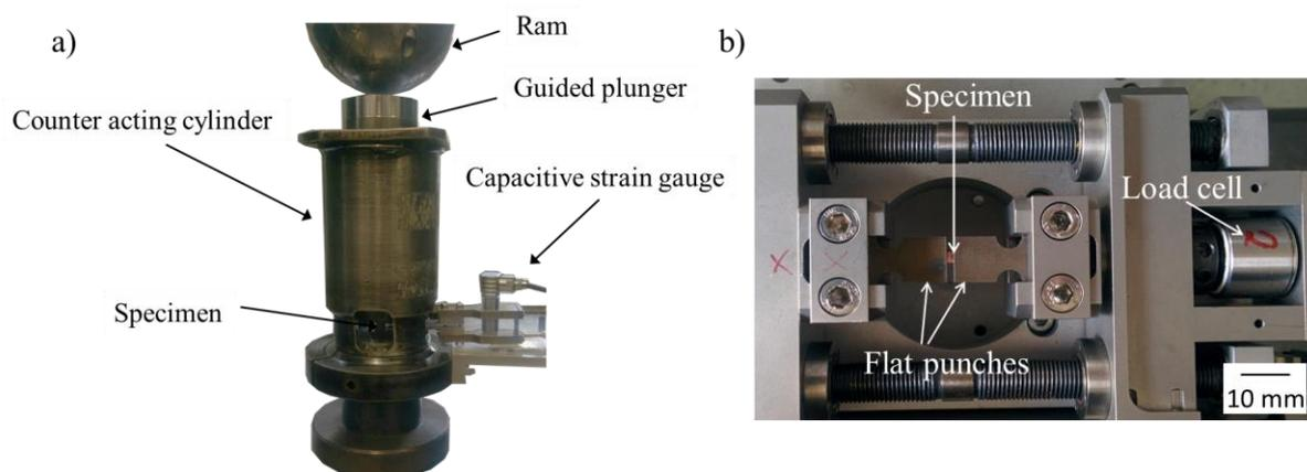
**Figure 1.** Experimental setup for a) compression tests and b) In situ SEM compression tests
