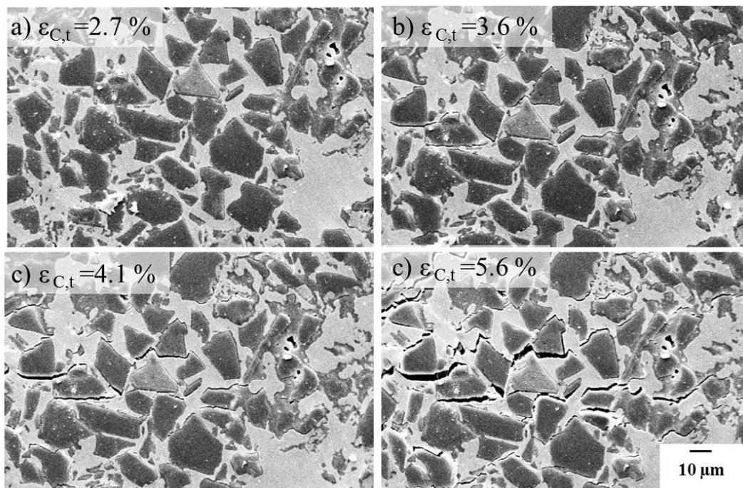
**Figure 5** Stress-compression diagram taken during the in situ compression test in the SEM (a-d: surface analysis)
