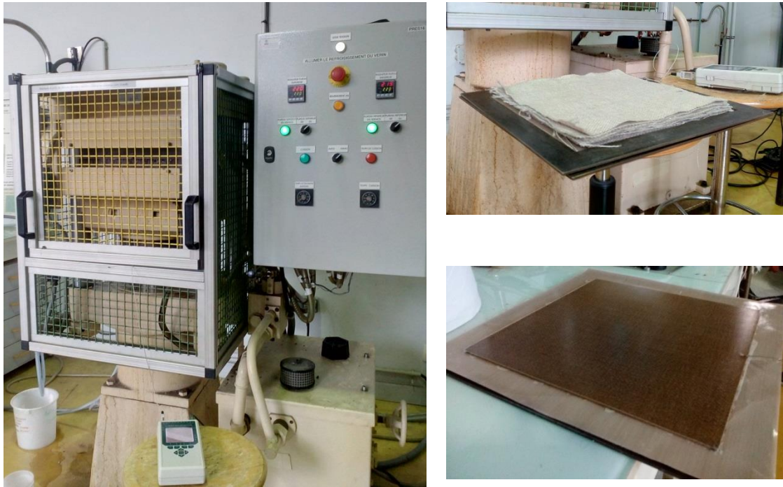
Figure 1. Manufacturing of the Flax-PP composite using thermopress
