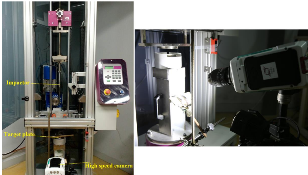
Figure 2. Drop tower setup used for low velocity impact testing
