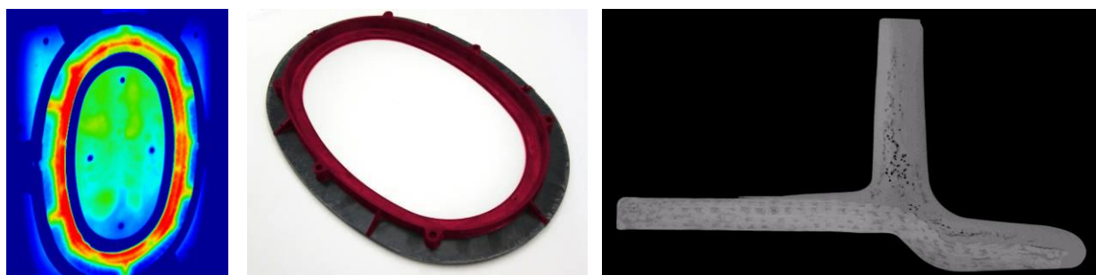
Figure 4. Pre-Heating of structural insert, Overmoulded WindowFrame, CT-Scan (f.l.t.r.)
