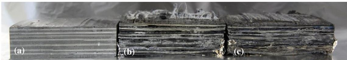
**Figure 2.** 29mm thick samples: (a) before being exposed to heat, (b) residue after 80 kW·m<sup>-2</sup> exposure for an hour (c) residue after 40 kW·m<sup>-2</sup> exposure for an hour.
