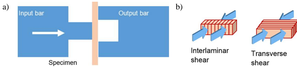
Figure 1: a) Principle of a punch SHB test, b) possible shear loading configurations [18].
