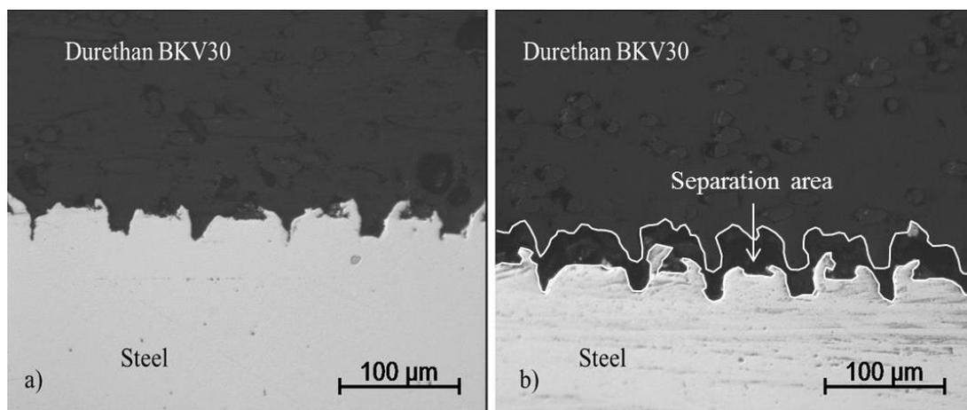
**Figure 7.** Separation of materials after specimen preparation: a) non-damaged specimen; b) specimen with pre-damaged interface
