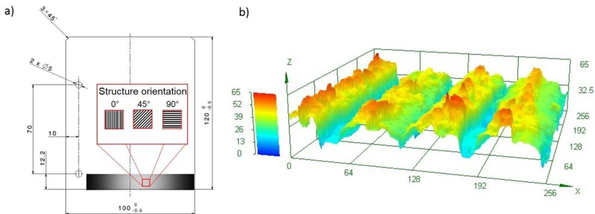
**Figure 1.** a) Schematic illustration of laser-structured specimens with detailed information about the varied structure orientation; b) laser scanning microscope image of laser-structured dual-phase steel
