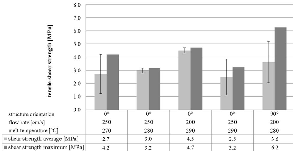
**Figure 6.** Tensile shear strength for Durethan BKV50 depending on manufacturing parameters
