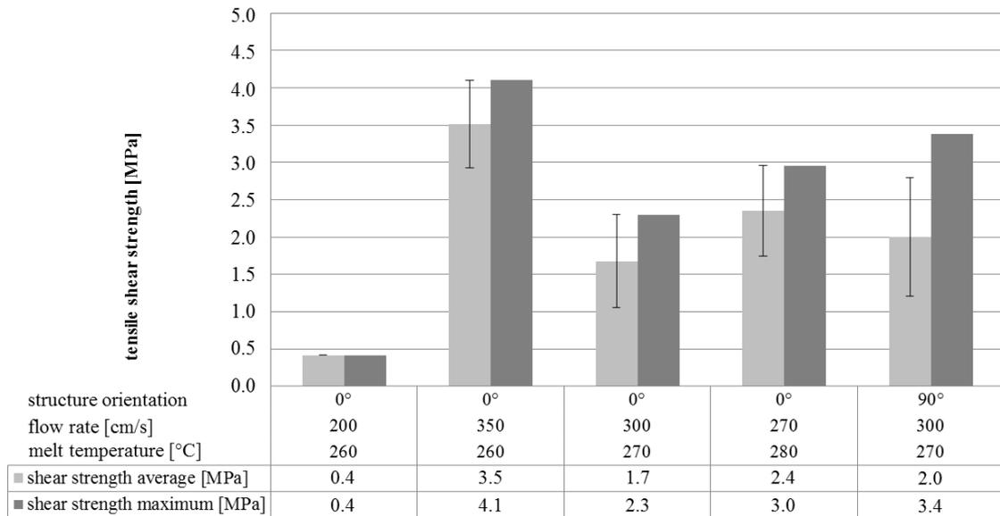
**Figure 4.** Tensile shear strength for Durethan B30s depending on manufacturing parameters
