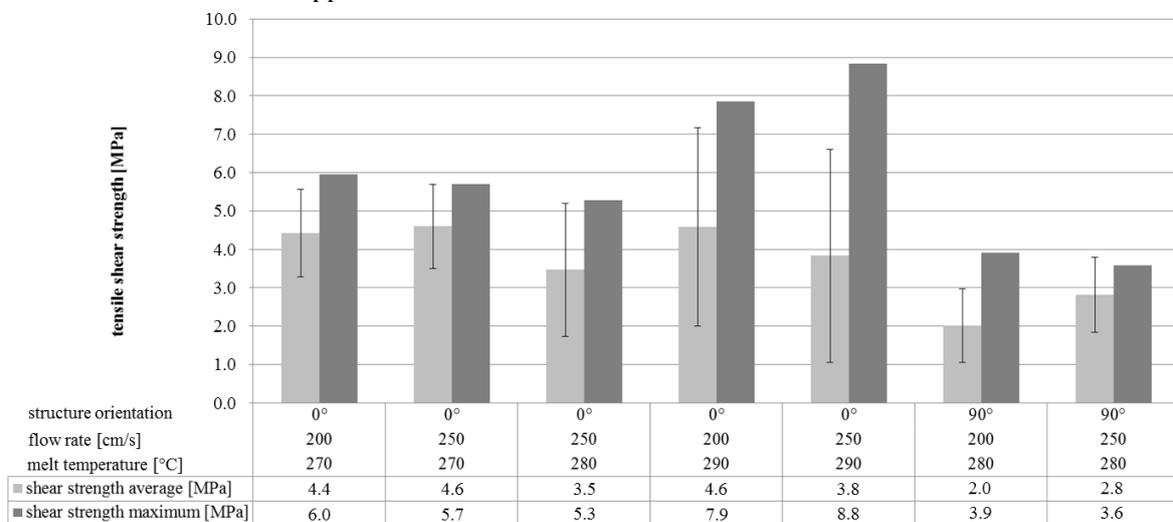
**Figure 5.** Tensile shear strength for Durethan BKV30 depending on manufacturing parameters
