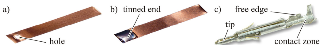
Figure 5. Different second contact partners: a) copper strip, b) tinned copper strip, c) crimping element
