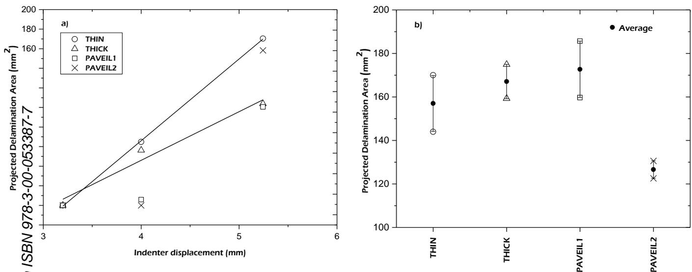
**Figure 1 C-scan projected delamination areas of a) indented and b) impacted specimens. The vertical bars highlight the dispersion between measurements**
