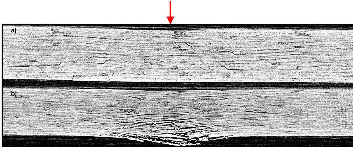
**Figure 3  $\mu$ CT cross-sections of a) THICK and b) THIN specimens impacted at 10 J. The arrow indicates the impacted point**
