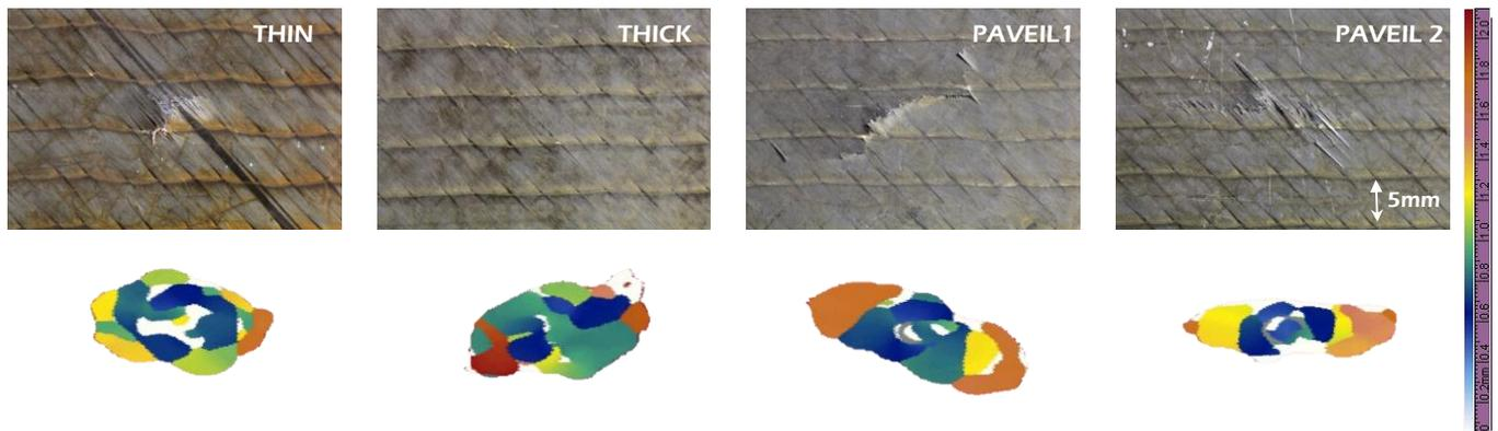
**Figure 2 Representative 10 J impacted specimens' back-face. Front face C-scan inspections are also plotted, where the colour scale represents different delamination depths (in mm). For interpretation of the references to colour in this figure legend, the reader is referred to the web version of this paper**
