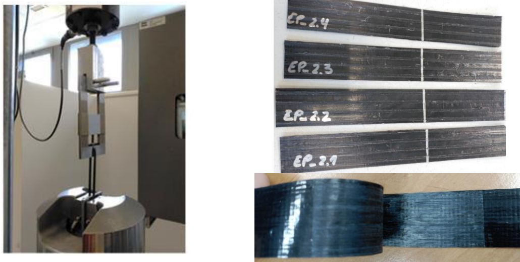
Figure 5 Samples at 2 m/min and laser power of 240W before and after testing
