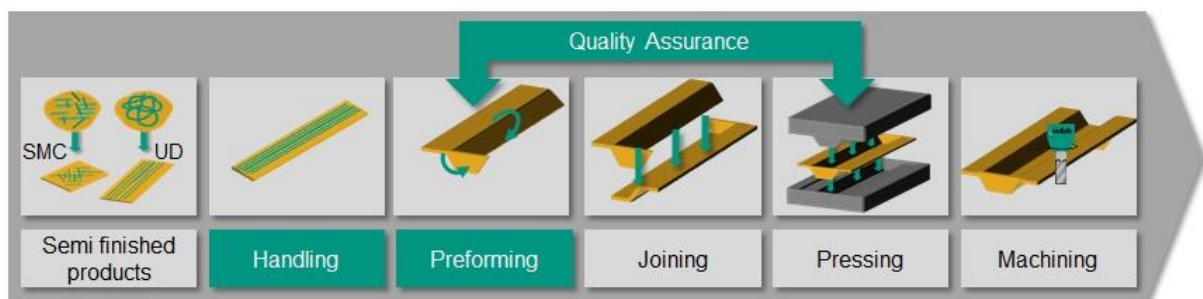
Figure 1. Process Chain of Part Manufacturing of the combined SMC-UD
