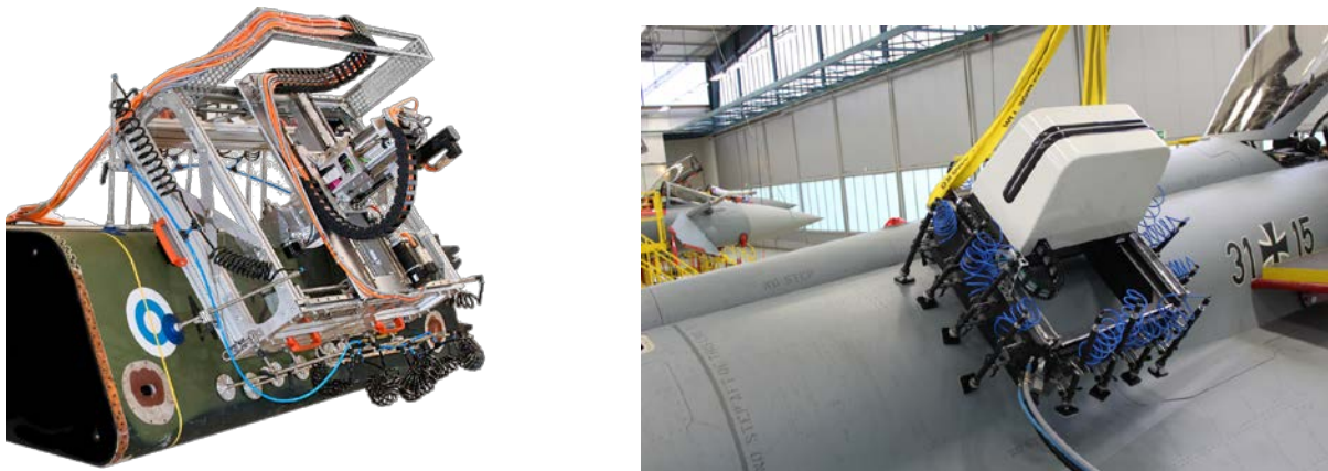
Figure 1. PM3 (left [1]) and FMRS (right) mounted on aircraft fuselage structures
