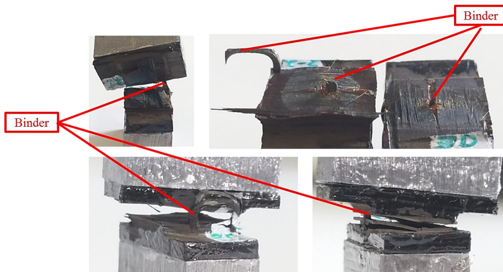
Figure 7: Images of failed 3DW coupons with all observed failure modes presented.
