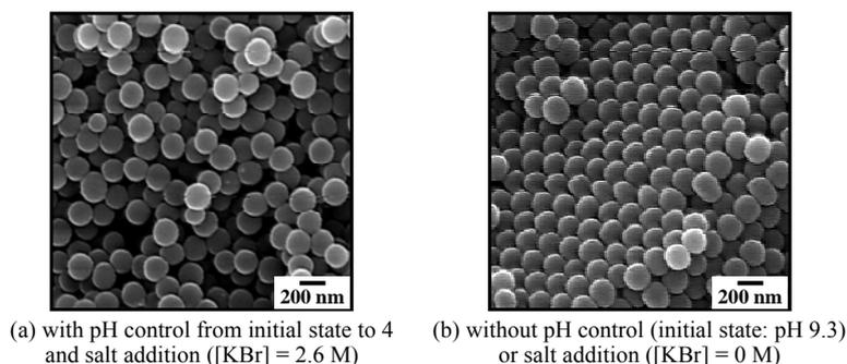
**Figure 3.** SEM micrographs showing arrangement structures of colloidal silica nanospheres in two types of agglomerates prepared from (a) silica sol solution with pH control and salt addition and (b) same sol solution without pH control or salt addition.
