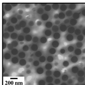
**Figure 5.** SEM micrographs showing an example of distribution of primary silica particles having hydrophilic surfaces with a diameter of 190 nm in epoxy resin highly filled with 34 % colloidal silica.
