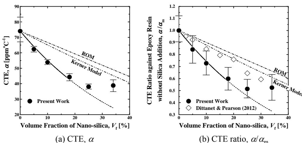
**Figure 8.** Effects of volume fraction of dispersed colloidal silica nanospheres on thermal expansion behavior of silica/epoxy resin nanocomposite fabricated using loose silica agglomerates dried under the standard condition: (a) Results of CTE values and (b) CTE ratio against epoxy resin without silica addition.
