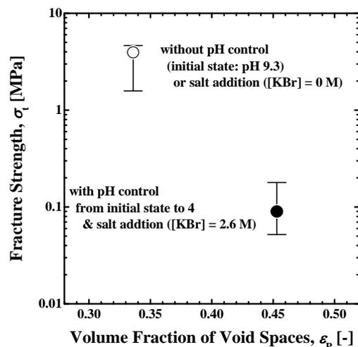
**Figure 4.** Relationship between fracture strength of prepared agglomerates of colloidal silica nanospheres and its void fraction.
