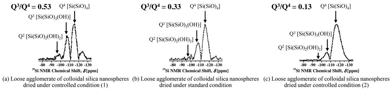
**Figure 6.**  $^{29}\text{Si}$  NMR (DD-MAS) spectra of loose agglomerates of colloidal silica nanospheres having different amounts of hydroxyl groups on their surfaces.
