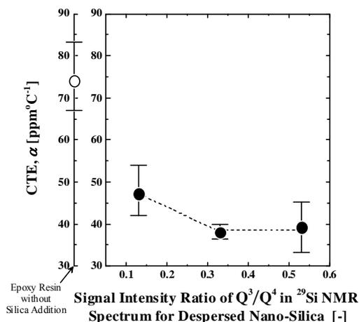
**Figure 7.** Relationship between coefficient of linear thermal expansion (CTE) of silica/epoxy resin nanocomposite fabricated for  $V_f$  being 25 % and amounts of hydroxyl groups on surfaces of colloidal silica nanospheres dispersed in epoxy resin matrix phase.
