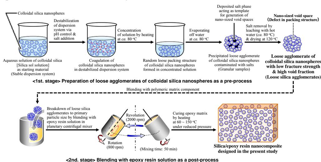
**Figure 2.** Process flow illustration for fabrication of silica/epoxy resin nanocomposite by solution-mixing method combined with process for pre-control of packing structure in agglomerates of silica nanospheres as inorganic fillers that enable acceleration of breakdown their agglomerates via blending with epoxy resin solution.
