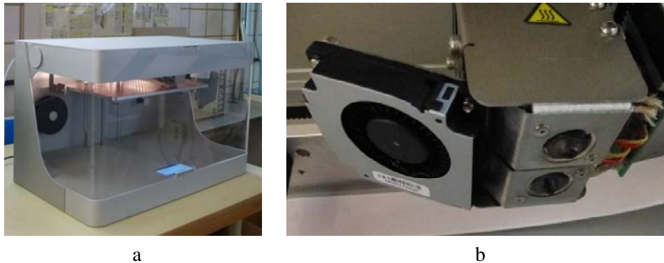
Figure 1. a) View of the 3D printer, b) Detail view of the two injectors of the printer.
