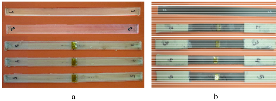
Figure 4. a) Glass fibre tensile test coupons, b) Carbon fibre tensile test coupons.
