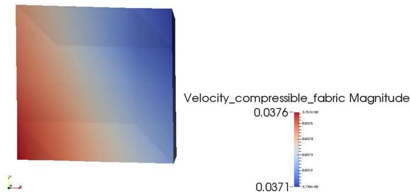
**Figure 5.** A top view a compressible fabric deformed by squeeze flow
