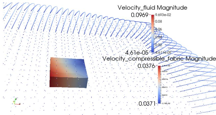
**Figure 4.** View of a compressible fabric inside a viscous domain (shown in dots)
