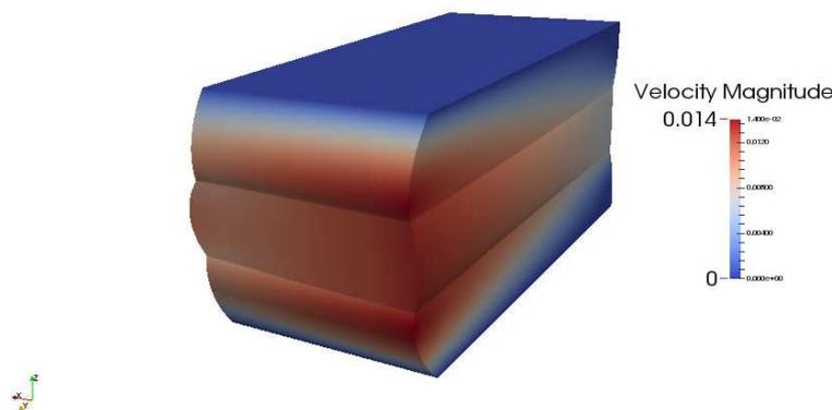
**Figure 2.** View of the deformed strands. The fiber orientation in the upper and lower strands is parallel to the  $x$ -axis, while in the middle one fibers align along the  $y$ -axis.
