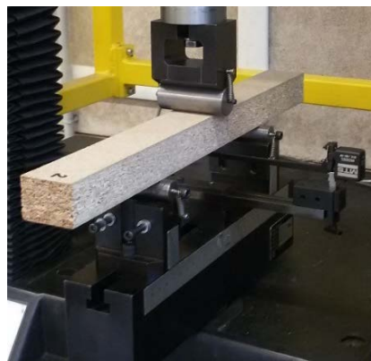
Figure 3: Three points bending set-up with variable span
